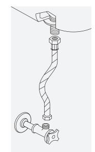
**A.** Connect the water supply line (not included) between the tank and shut-off valve.
