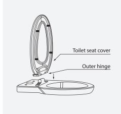
3. Get the seat cover and outer hinge ready, then, assembled the outer and inner hinge in place.
