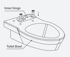
2. Align the inner hinge with toilet bowl's hole and insert screws to make the inner hinge fixed.
