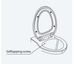
4. Lift the seat cover up, put the selftapping screws into composite hole and tighten them up.
